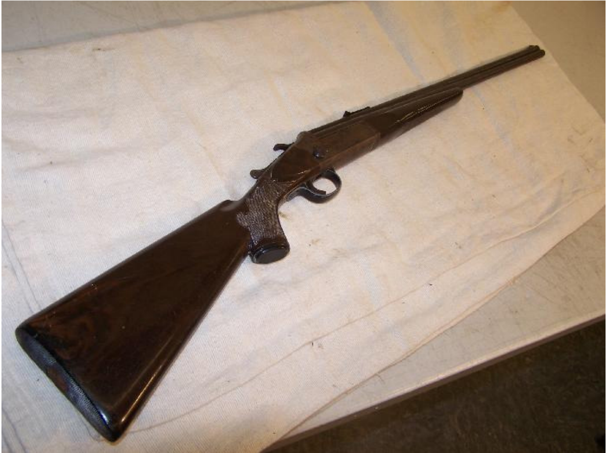
Typical Stevens .22 caliber, .410 caliber Over/Under Long gun.
